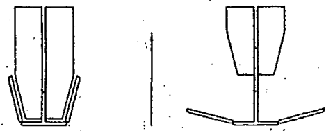
Drain anchor is fixed to the drain up, prevents soil from intruding into the mandrel during drain installation and keeps the drain in place when the mandrel is withdrawn.
